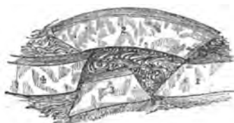
DISLOCATION OF A BED OF SANDSTONE, STATE'S PRISON QUARRY.
