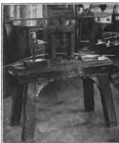
FIRST COINING PRESS. Primitive device used in 1795 for making United States coins.
