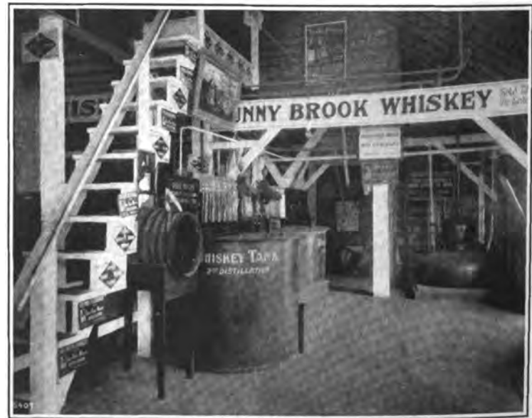
INTERIOR VIEW OF THE MODEL SUNNY BROOK DISTILLERY, Showing Doubler and First and Second Distillation Tanks.
