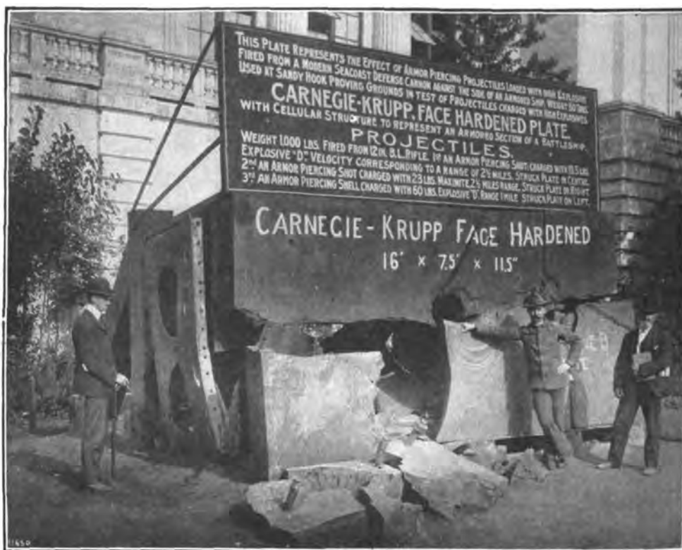
NAVY DEPARTMENT EXHIBIT—ARMOR-PLATE TESTS.
